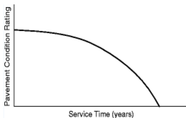
Figure (1): typical pavement performance curve
